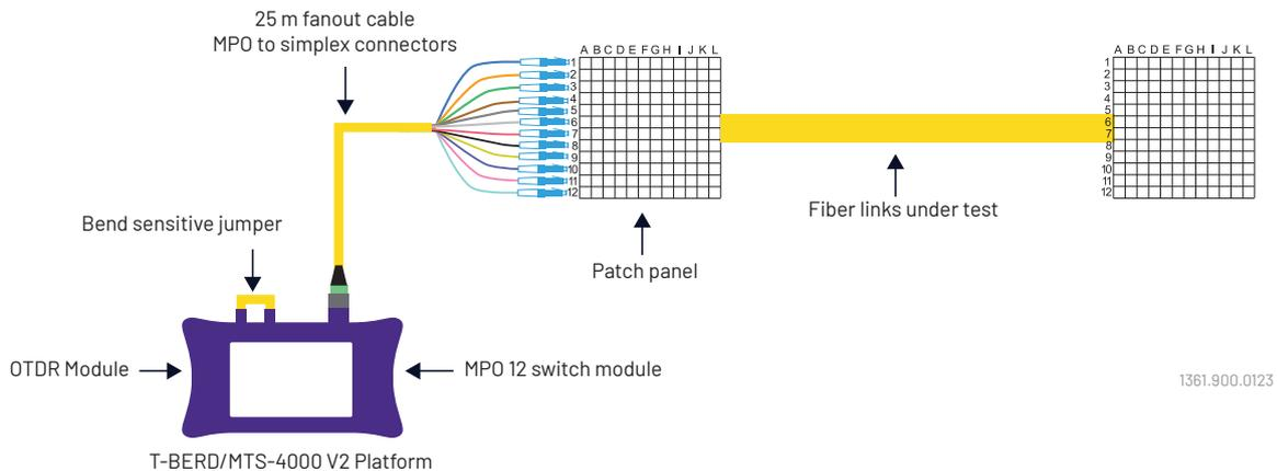
An onboard MPO based switch module with fanout/breakout cable for bulk certification of simplex fibers
